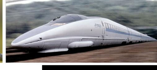
ABOVE: Biomimicry in action. Engineers seeking to decrease the pressure shock waves produced by bullet trains as they entered and exited contained air in tunnels looked to the form of the Kingfisher bird, which has a beak and head designed to smoothly penetrate the water's surface in a high speed dive. The result? A 10% increase in train speed, at the same time as a 15% decrease in power needed to propel the trains.
