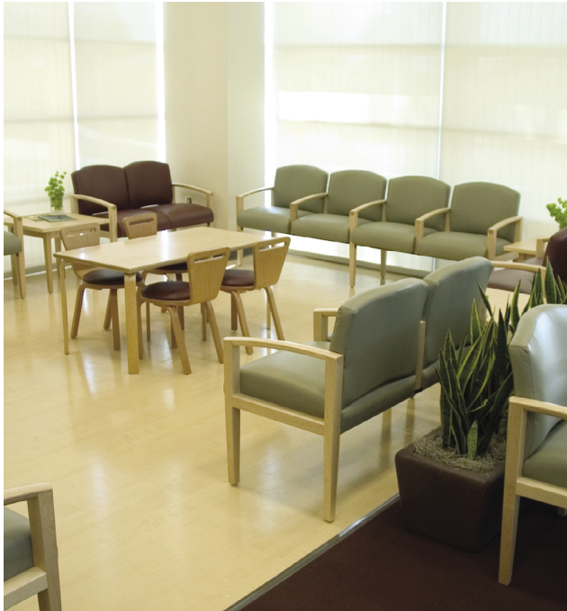
The use of 12-foot glazing in the waiting area eliminates the need for artificial lighting during most business hours.
